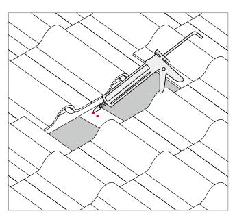
2. Position hook, Drill 2 pilot holes at the center of the rafter, and backfill with sealant.
