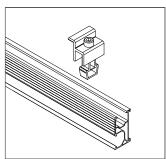
**3.** Place last module in position on rail with a minimal 50mm from rail end, slide end clamps onto both rails and tighten the screws to secure the PV module.
