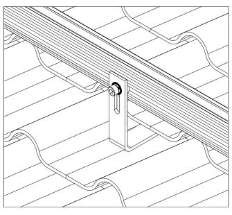
4. Connect rails to tile hook to 16 N·m using a 6mm Allen key or hex driver bit
